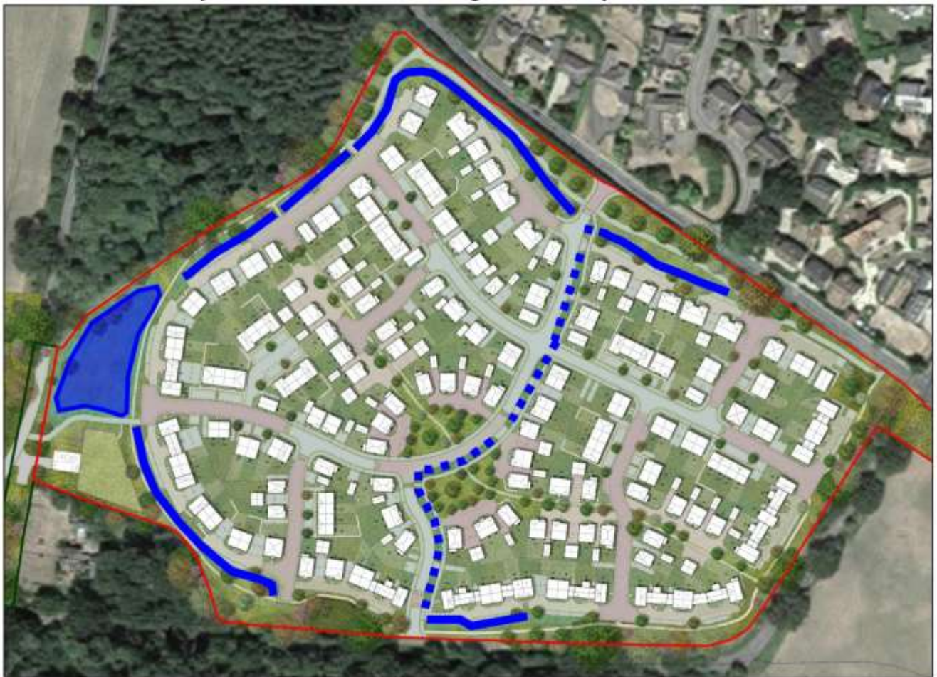
figure 19: Location of attenuation basin and swales
